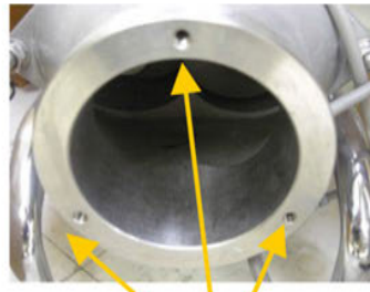
There are 3 holes on the pugmill nozzle where the die will be attached
