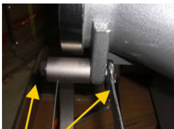
1. Take off the original nut and bolt that holds the clay cutter on the front of the nozzle
