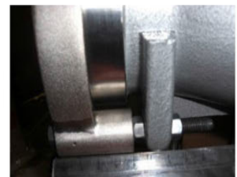
2. Place the M8 x 75 mm (or longer), full thread bolt through the clay cutter. Then thread the M8 nut into the bolt. This will create a space between the clay cutter and mounting bolts of the die. Mount the clay cutter onto the nozzle and tighten the bolt to secure.
