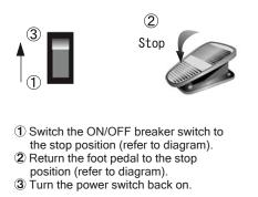
Note: If the pedal is not returned to the stop position before the power switch is turned on, the wheelhead will not turn; your wheel will not respond.
